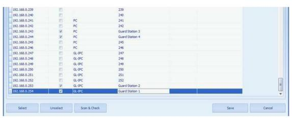
If all the device has been installed in the project, you can click the Scan & Check button to search if the selected IP Nodes are online. If not installed yet, click Save button to write the info to the database. Then main interface will show the devices like the following picture.
