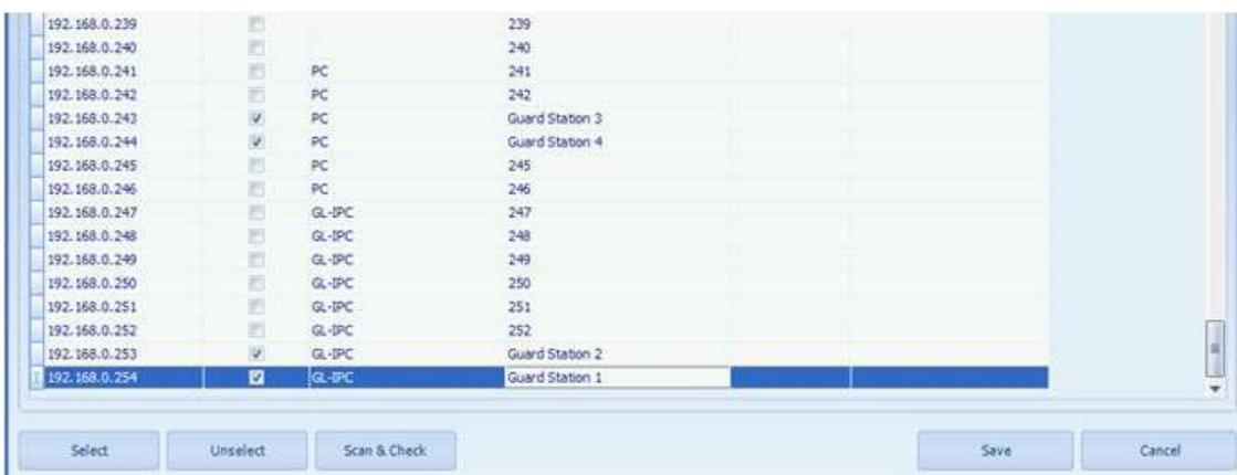
If all the device has been installed in the project, you can click the Scan & Check button to search if the selected IP Nodes are online. If not installed yet, click Save button to write the info to the database. Then main interface will show the devices like the following picture.
