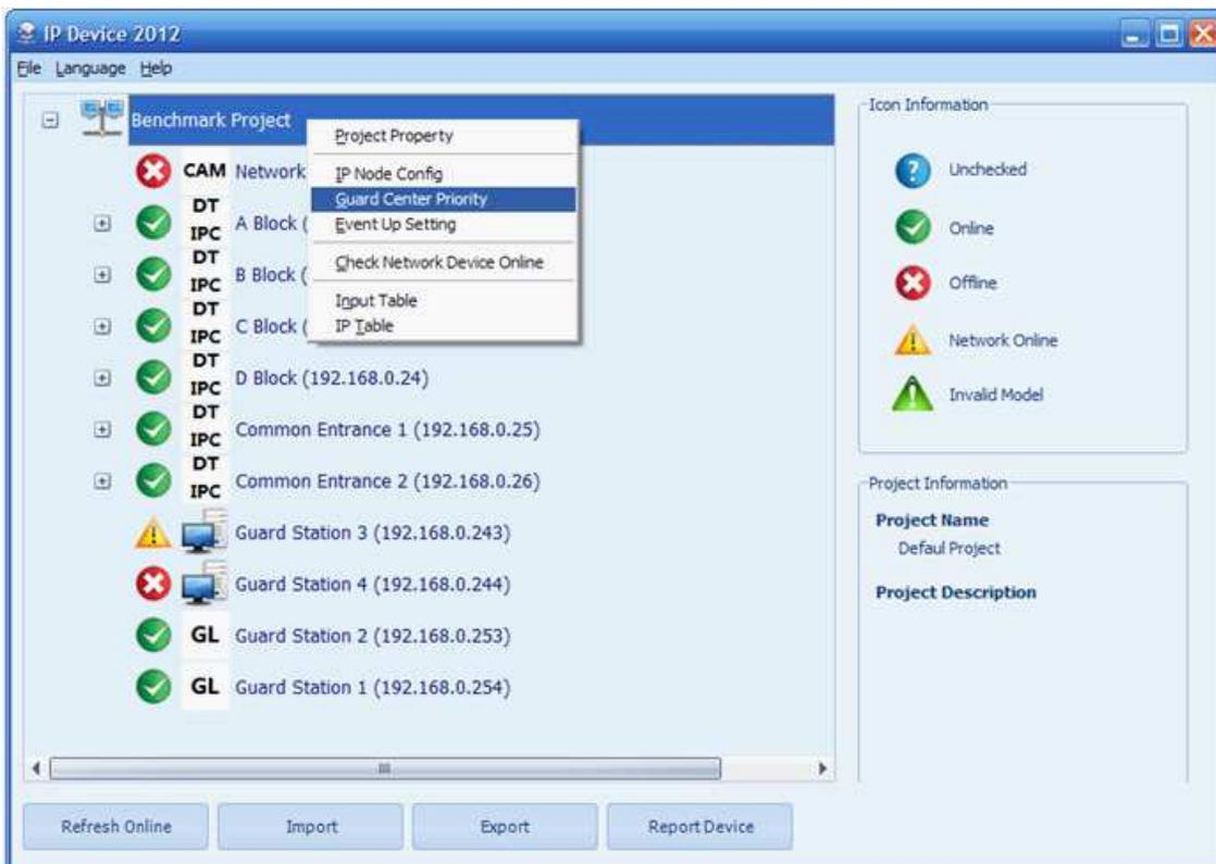
See the following picture, there are 8 position for calling transfer. For example, when one door station or monitor call Guard Centre, it will call GL 1 firstly, if GL 1 is busy or offline, the calling will be diverted to GL2, if GL2 is busy or offline, the calling will be diverted to GL 3... Repeat this till divert the calling to the last Guard Centre.
