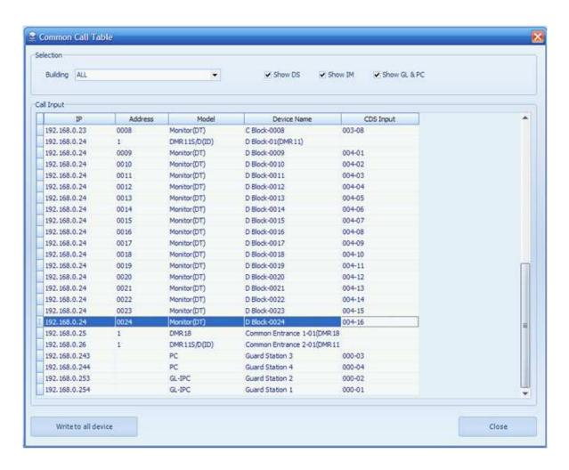
As the above CDS Input, for example, press 004-07 to call the monitor whose user code is 15 in D block after the rules are download to device.
