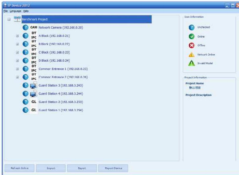
As you see, D Block, Guard Station 2 & Guard Station 1 are offline. Network Camera is online, but device model doesn't correspond with the connected device. Other devices is normally online.
