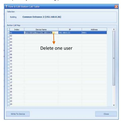
Fulfill the call table, then press Write To Device to download the info to the corresponding DT-IPC. You can call user or Guard Center by the corresponding button, for example, press 32nd button to call Default Guard Center, press 20th button to call the monitor whose user code is 15 in D block.
