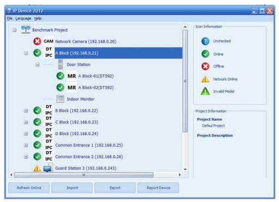
Monitor Config: Click the right mouse button on A Block -> Select Monitor Config on the pop-up window -> Config just like the following picture -> Click Save button to confirm -> Software will check if the monitors are online automatically.
