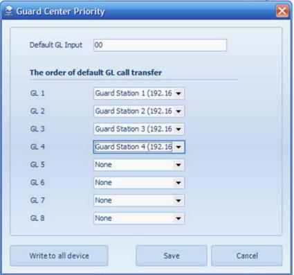
Press the Write to all device button to download the info to all devices connected to the network, and info will be saved to database at the same time. If only press Save button, the info just is kept in the database, isn't downloaded to devices.
