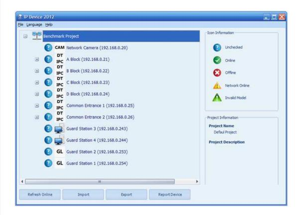
If you want to check if the devices are online, you can press Refresh Online button or click right mouse button on Benchmark Project then select Check Network Device Online. See the following picture, Means device offline, and means PC is online, but IP-Agent isn't opened. indicates the model of IP Node is wrong selected, or wrong DIP switch setting of IPC.
