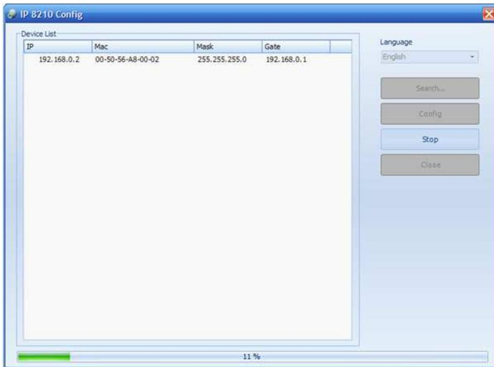
e. Select the device in the Device List frame, then press Config button
