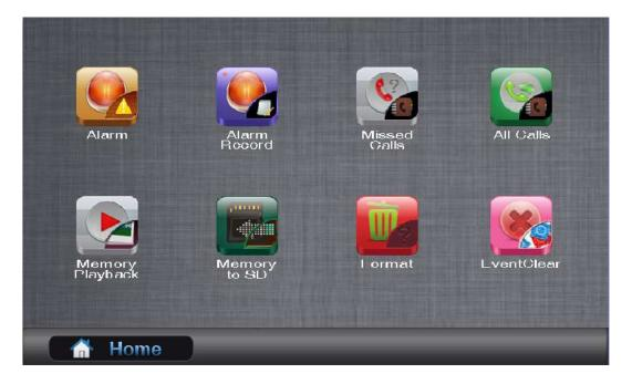
The G21 supports picture memory function, and the pictures can be playbacked on G21, at this page ,press **Memory Playback** icon ,each memo can display 4 pictures named by date, and the pictures can be copied to SD card, just press **Memory to SD** icon.
