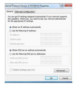
\* Input IP address, Subnet mask and Default gateway as following picture shows, then press OK button to finish setup
