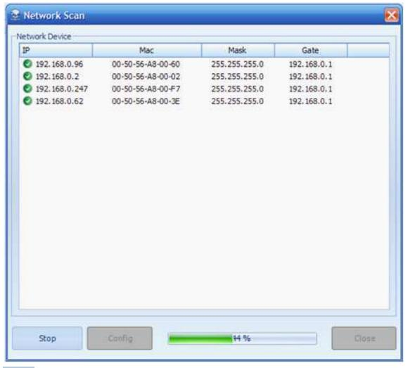
h) Double click 192.168.0.2, then a window pops up for modifying IP, input 93 then Mac address will be automatically modified. Press OK button to confirm modification.
