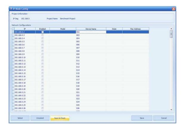
g) Then it will pop up a window to show devices that are detected. Assume that 192.168.0.2 is the device that is supposed to be set to 192.168.0.93.
