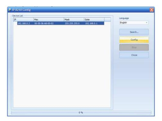
f. It will pop up a window for IP address config. Modify IP address, and then press OK button to confirm. Its Mac address will be automatically modified simultaneously.
