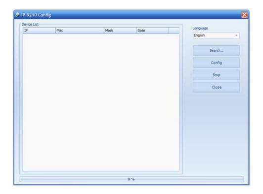
d. Press Search... button to search the device. You can press Stop button to end the search after the device has been detected. Just like the following picture shows
