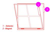
Tilt detector detects the vertical deviation of the device relative to the initial position of more than 5°. DoorProtect Plus can be installed on windows including dormer windows, and the system can be armed, when they are in the airing mode (you should previously disable the magnetic sensor in the settings).
