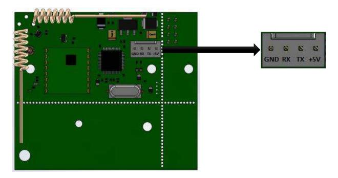
Speed for connection through UART interface - 57600 bit/s
