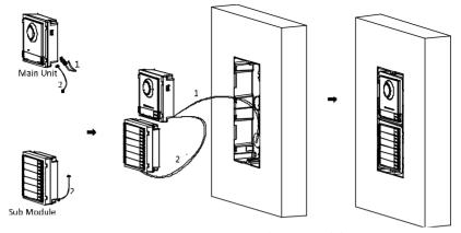
Figure 4-27 Connect Wires and Insert Modules
