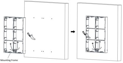
Figure 4-47 Fix the Mounting Frame
