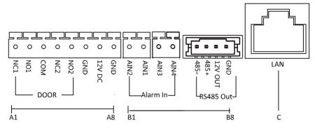
Figure 3-1 Terminals and Interfaces
