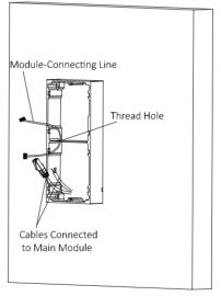
Figure 4-17 Placement of Lines
