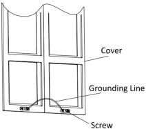
Figure 4-64 Connect the Grounding Line to the Cover
