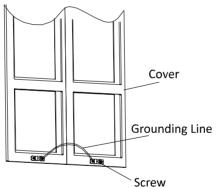
Figure 4-51 Connect the Grounding Line to the Cover
