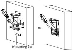
Figure 4-11 Remove the Mounting Ears
