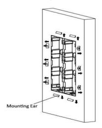
Figure 4-60 Remove the Mounting Ears
