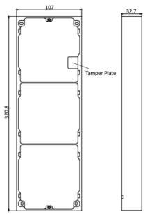
Figure 4-44 Front and Side View
