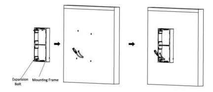
Figure 4-16 Fix the Mounting Frame
