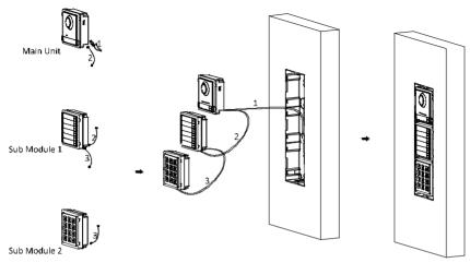
Figure 4-42 Connect Wires and Insert Modules
