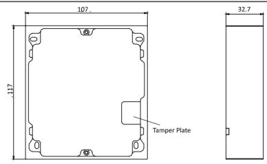
Figure 4-1 Front and Side View
