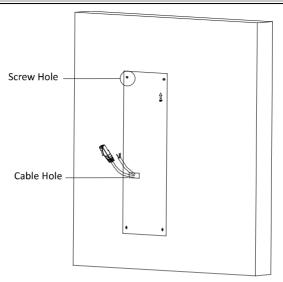
Figure 4-30 Chisel Screw Hole
