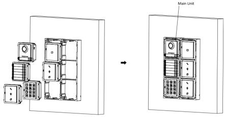
Figure 4-50 Insert the Modules
