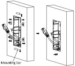
Figure 4-26 Remove the Mounting Ears
