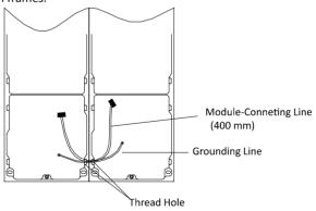
Figure 4-46 Place the Grounding Line and Module-Connecting Line
