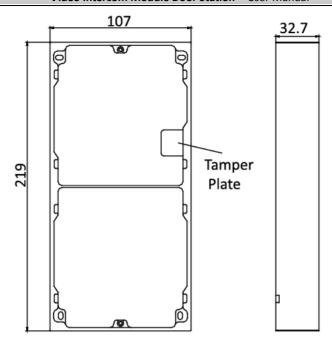
Figure 4-14 Front and Side View
