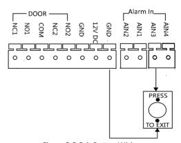
Figure 3-5 Exit Button Wiring
