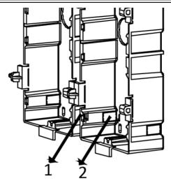
Figure 4-57 Remove the Plastic Sheets
