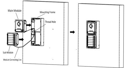
Figure 4-19 Insert the Modules
