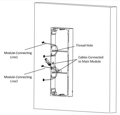
Figure 4-32 Placement of Lines
