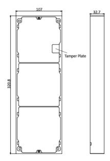
Figure 4-29 Front and Side View
