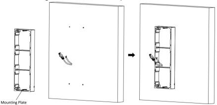
Figure 4-31 Fix the Mounting Frame
