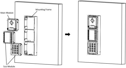
Figure 4-34 Insert the Modules
