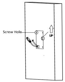
Figure 4-15 Chisel Screw Hole
