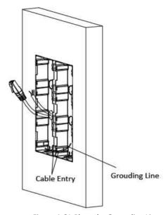
Figure 4-61 Place the Grounding Line
