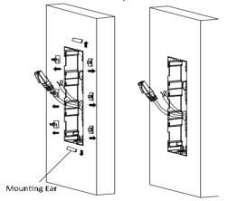
Figure 4-41 Remove the Mounting Ears
