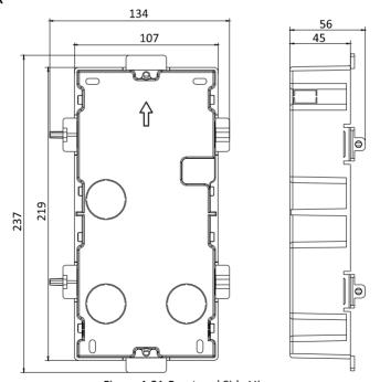
Figure 4-21 Front and Side View
