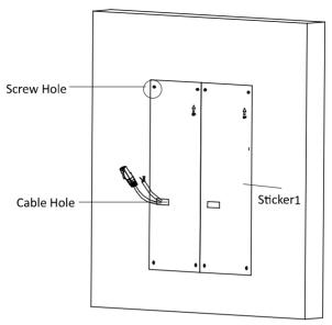
Figure 4-45 Chisel Screw Hole
