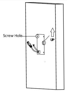
Figure 4-2 Chisel Screw Hole
