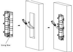
Figure 4-39 Mark the Screw Holes
