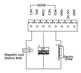
Figure 3-3 Door Lock Wiring
