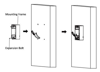
Figure 4-3 Fix the Mounting Frame
