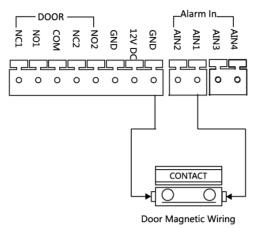
Figure 3-4 Door Magnetic Wiring
