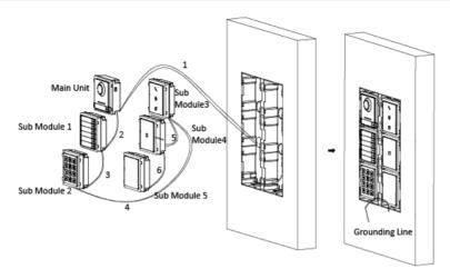
Figure 4-62 Install Mounting Frames
